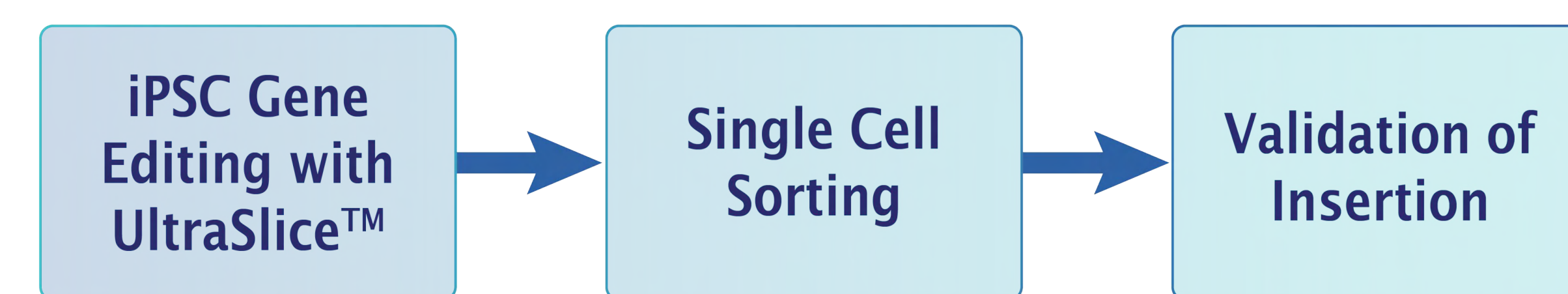
Figure 1. Flow chart illustrating the process of gene-edited iPSC cell line development. The iPSCs are first electroporated using mRNA encoding UltraSlice™, Factor Bioscience's proprietary gene-editing technology, to insert a single-stranded DNA (ssDNA) repair template for a gene of interest. Gene-edited iPSCs are then single-cell sorted using a microfluidic cell sorter. When single-cell derived colonies recover, biallelic insertion is confirmed by agarose gel electrophoresis and amplicon sequencing.
